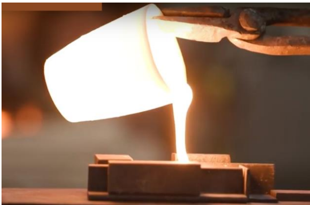
Creating simulant radioactive waste glass in the laboratory, in preparation for groundwater leaching tests. Credit: Claire Corkhill
